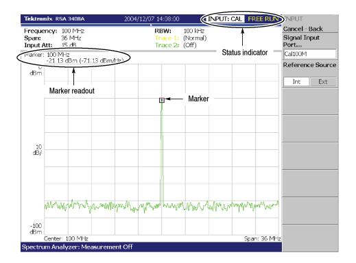
Figure 1-1: Spectrum of the calibration signal (100 MHz, -20 dBm)
