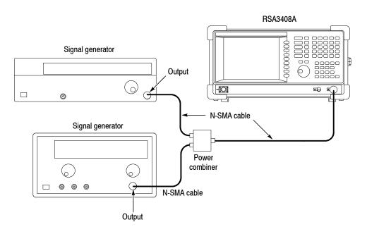
**b.** Connect the power combiner output through a 50  $\Omega$  N-SMA coaxial cable to the analyzer **INPUT**.
