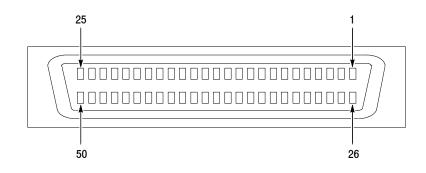
Figure 2-2: Digital IQ output connector pin assignment
